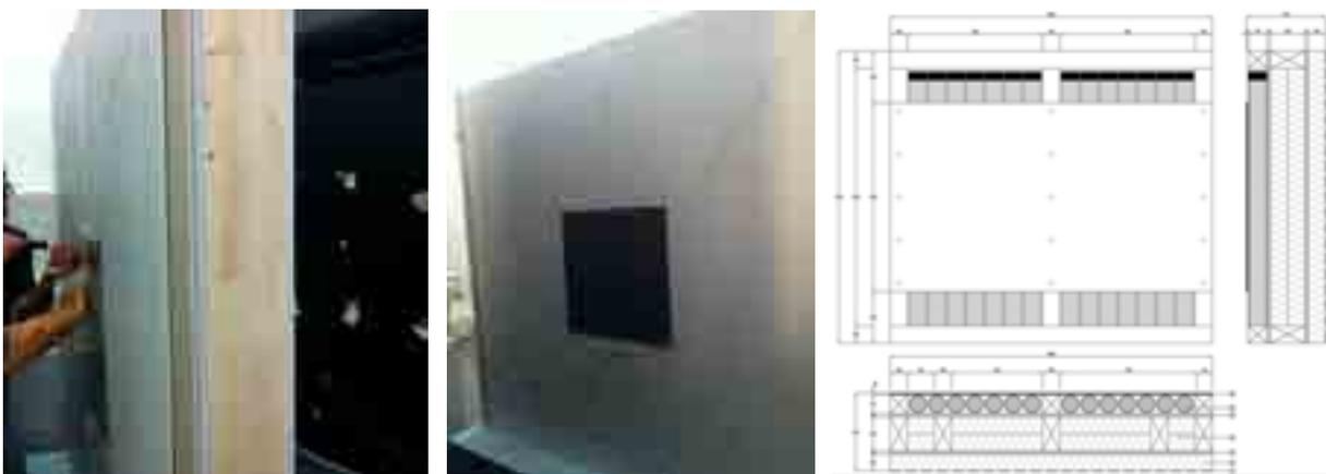
Figure 1 - Wall prototype made by aluminium pipes ready for the hot box tests
