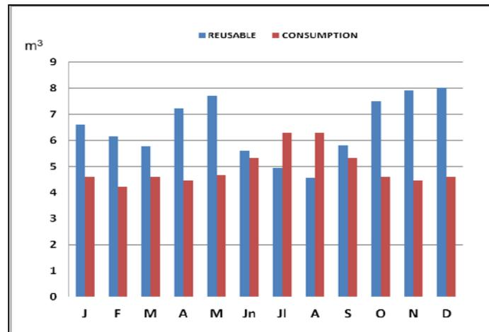
If it is made an annual analysis the water balance is positive, that means that it is possible to cover the house needs with the water storage of the months with surplus. So that, depending on pluviometry Casa Pi can be self-sufficient.
