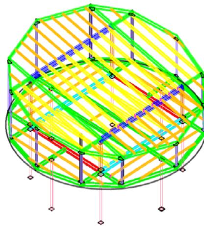
In order to facilitate assembling in time, and the availability of space in the solar village as security definitions, the structure was designed in such way so that the overall shape of the polygonal circle was decomposed into semicircular modules. These will come welded from the factory, having only to make the connections between them during the assembly, minimizing the amount of bolted unions in order to facilitate the assembly.
